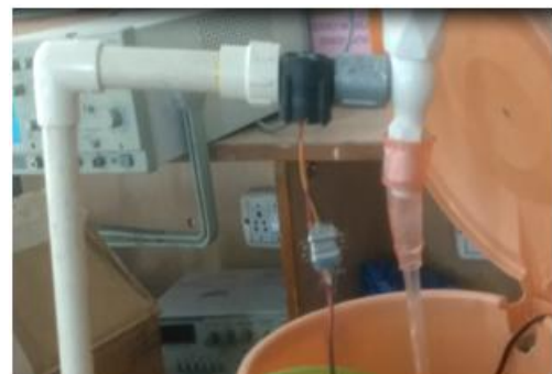
Fig b: Water flowing through tap across the flow meter
