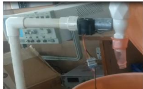
Fig a: flow meter connected to the tap
