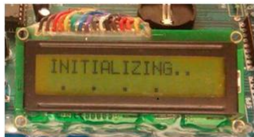
Step1: initializing the LCD
