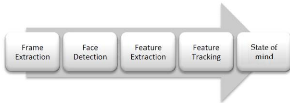
Figure 2: Image processing flow for a single image.
